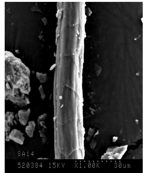
Elliptical Suri Fiber – MSF 5.25. About 30% of the alpaca samples had one or two grooves running along the surface of the fiber, indicating they are probably elliptical rather than round.
