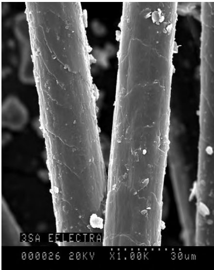
MSF 5.0 Suri is nearly as bright as mohair but has a much lower AFD.
